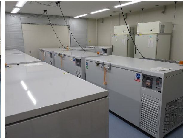
-80°C deep-freezer for frozen samples (7 units)
