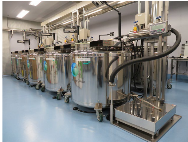
Liquid nitrogen tanks (15 units in vapour phase, 1 unit in liquid phase) for frozen samples
