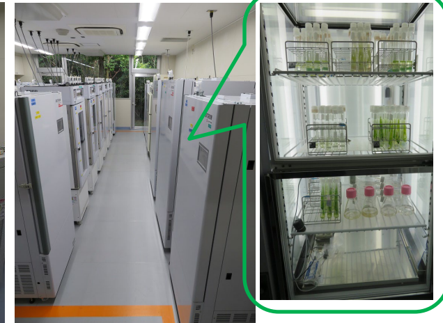
Plant growth chamber for active cultures (28 units)
